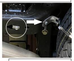
4. Relocate the factory spare tire cable bracket to ten hole closer to the spare tire using bolt kit #L. You can install the passenger side overaxle pipe. Note all hangers will sit in the rubber hangers' level.
