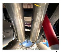
3. Install supplied 3½" clamp #H onto inlet end of new muffler #B and slip onto end of the head pipe with 2-1/4" inserted into muffler. Muffler outlets will sit level. Tighten with allowance for adjustment.
