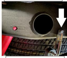
5. Install the Driver side hanger into the factory existing hole in frame. Install the Driver side pipes. Keep everything loose until everything is installed.
