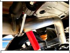
5. Be sure you have adjusted the tailpipe in the position to receive maximum clearance from both spare tire and shock. Do not tighten
