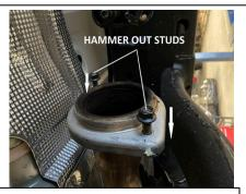
2. First you'll need to unbolt the factory flange and remove the exhaust. Next, hammer out the studs protruding from the factory flange, then install head pipe #A and tighten with allowance for adjustment using Bolt Kit #F
