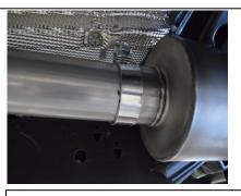
3. Install supplied 3½" clamp #H onto inlet end of new muffler #B and slip onto end of the head pipe with 2-1/4" inserted into muffler. Tighten with allowance for adjustment.
