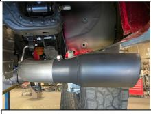
6. With proper clearance from spare tire, install the exhaust tip onto the tailpipe. The system was designed to have the tip 1" below the quarter panel of the vehicle. With the tip in your desired position begin to tighten down all clamp connections from front.
