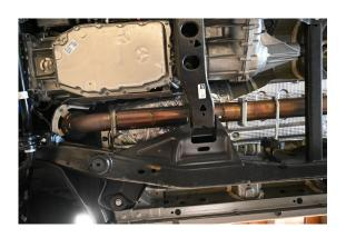
2. Install headpipe #a and #b onto stock pipe using factory hardware and clamp #g. Insert welded hanger into rubber grommet. (do not tighten.)
