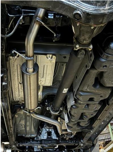
**3.** INSTALL MUFFLER **#B** ONTO HEAD PIPE 1-1/2" TO 2" WITH THE LOUVERS FACING TOWARDS THE CONVERTER. THEN INSTALL OVERAXLE **#C** USING CLAMP **#F**. USE A JACK STAND TO SUPPORT THE MUFFLER. (DO NOT TIGHTEN)
