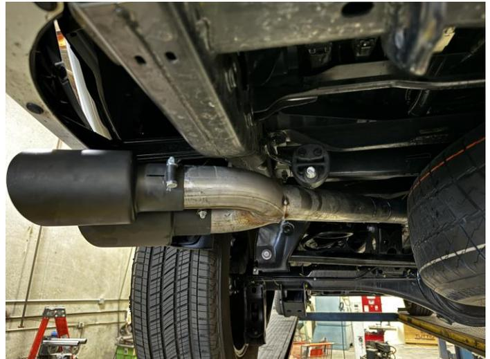
**4.** LASTLY, INSTALL EXIT PIPE **#D** USING CLAMP **#F**. INSERT WELDED HANGER INTO RUBBER GROMMET. (ONCE DESIRED LOCATION IS ACHIEVED WITH TIPS **#E** INSTALLED, BEGIN TIGHTENING ALL CLAMPS STARTING FRONT TO BACK.)
