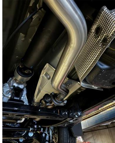
**2.** INSTALL HEAD PIPE **#A** ONTO YOUR EXISTING STOCK 2-BOLT FLANGE AND SECURE. Use clamp hanger **#H** to attach headpipe to rubber grommets (DO NOT TIGHTEN). (DOUBLE CAB LONG BED WILL NEED TO USE HEADPIPE EXTENSION **#G** WITH BAND CLAMP **#F**)
