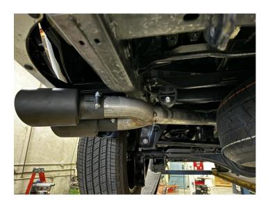
**4.** LASTLY, INSTALL EXIT PIPE **#D** USING CLAMP **#F**. INSERT WELDED HANGER INTO RUBBER GROMMET. (ONCE DESIRED LOCATION IS ACHIEVED WITH TIPS **#E** INSTALLED, BEGIN TIGHTENING ALL CLAMPS STARTING FRONT TO BACK.)
