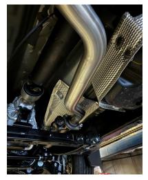
2. INSTALL HEAD PIPE #A ON TO YOUR EXISTING STOCK 2-BOLT FLANGE AND SECURE. INSTALL CLAMP HANGER G ONTO HEADPIPE. INSTALL EXTENSION PIPE IF REQUIRED. DO NOT TIGHTEN UNTIL THE END
