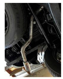
**4.** LASTLY, INSTALL EXIT PIPE **#D** USING CLAMP **#F**. INSERT WELDED HANGER INTO RUBBER GROMMET. (ONCE DESIRED LOCATION IS ACHIEVED WITH TIP **#E** INSTALLED, BEGIN TIGHTENING ALL CLAMPS STARTING FRONT TO BACK.)
