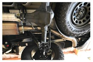
**4.** INSTALL OVERAXLE PIPE **#D** INTO MUFFLER  $1\frac{1}{2}$ " TO 2". INSERT HANGERS INTO RUBBER GROMMETS, USE CLAMP **#E** TO SECURE PIPE TO MUFFLER (DO NOT TIGHTEN).
