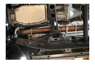
2. INSTALL HEADPIPE #A AND #B ONTO STOCK PIPE USING FACTORY HARDWARE AND CLAMP #E. INSERT WELDED HANGER INTO RUBBER GROMMET. (DO NOT TIGHTEN.)
