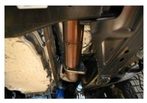
1. TO REMOVE YOUR STOCK EXHAUST, UN-BOLT IT FROM THE FLANGE THEN REMOVE HANGERS FROM RUBBER GROMMETS BY PULLING EXHAUST TOWARDS THE REAR OF THE VEHICLE, USE WD-40 TO AID IN REMOVAL, LEAVE GROMMETS IN PLACE.
