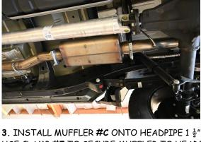
3. INSTALL MUFFLER #C ONTO HEADPIPE 1  $\frac{1}{2}$ " TO 2". USE CLAMP #E TO SECURE MUFFLER TO HEADPIPE. DO NOT TIGHTEN. USE A JACK STAND TO HOLD UP THE MUFFLER.
