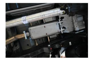
**3**. Install muffler #c onto headpipe  $1\frac{1}{2}$ " to 2". Use clamp #g to secure muffler to headpipe. Do not tighten. Use a jack stand to hold up the muffler.
