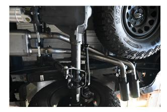
**4**. Install passenger side # D & driver side tailpipe #E into muffler  $1\frac{1}{2}$ " to 2". Insert hangers into rubber grommets, Use clamps #h to secure pipes to muffler (do not tighten) and use bolt kit #i to secure tailpipes to each other.
