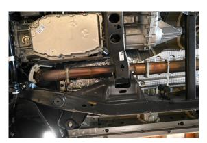
2. Install headpipe #a and #b onto stock pipe using factory hardware and clamp #g.
