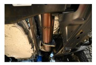
1. To remove your stock exhaust, un-bolt it from the flange then remove hangers from rubber grommets by pulling exhaust towards the rear of the vehicle, use wd-40 to aid in removal, leave grommets in place.
