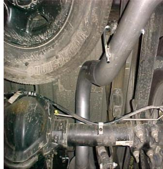
NEXT, INSTALL OVERAXLE TAILPIPE # D INTO MUFFLER 1-1/2" - 2". USE CLAMP # I TO SECURE PIPE TO MUFFLER, DO NOT TIGHTEN.
