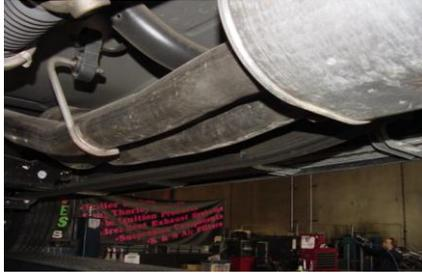
TO REMOVE STOCK EXHAUST, CUT 13" FROM THE FRONT OF THE MUFFLER, MEASURE TOWARDS THE FRONT OF THE VEHICLE. LEAVE ALL RUBBER GROMMETS ON THE HANGER. USE WD-40 TO AID IN THE REMOVAL OF EXHAUST AND HANGERS. SUPPORT THE CATALITIC CONVERTER BEFORE CUTTING.
