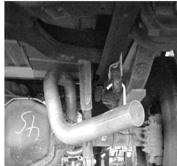
5. INSTALL OVERAXLE TAILPIPE # C INTO THE OUTLET OF THE MUFFLER 1 1/2" TO 2". INSERT THE REAR WELDED HANGER INTO THE FACTORY RUBBER GROMMET. USE CLAMP #E TO ATTACH THE OVERAXLE PIPE TO THE MUFFLER OUTLET. DO NOT TIGHTEN. INSTALL EXIT PIPE # D AND ATTACH USING CLAMP #E.
