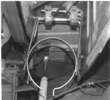
3. INSTALL BAND CLAMP #H AND INSERT RODS INTO RUBBER GROMMETS LOCATED JUST ABOVE THE AXLE AND ATTACH WITH BOLT KIT # I.
