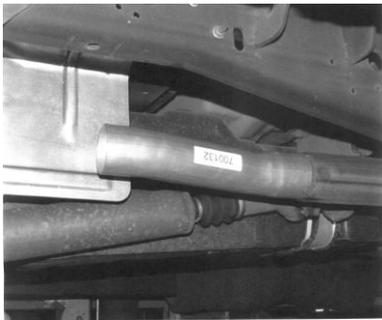
2. INSTALL HEADPIPE #A ONTO THE FACTORY EXTENSION PIPE. USE CLAMP #E TO ATTACH IT TO THE FACTORY EXTENSION PIPE. DO NOT TIGHTEN
