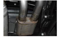
Install head pipe # A Use a jack stand to support the factory exhaust.
