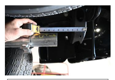
**3)** THIRD, CUT PASSENGER SIDE OUTLET PIPE 6" FROM THE REAR LEAF SPRING MOUNTING BUCKET
