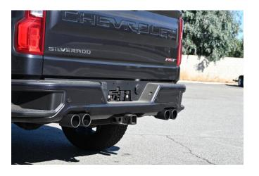
4) FINALLY, ADJUST TIPS TO DESIRED LOOK AND DEPTH THEN TIGHTEN. NOTE: THESE TIPS HAVE AN EXCEPTIONAL AMOUNT OF DEPTH ADJUSTMENT
