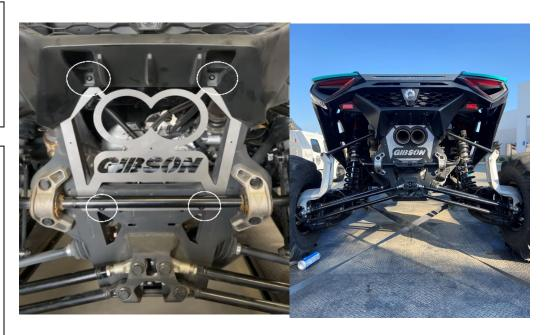
"MAKE SURE YOU HAVE A 1" CLEARANCE ON ALL PIPES FROM ALL RUBBER BRAKE LINES, SHOCK BOOTS, TIRES, ETC..." TORQUE ALL CLAMPS TO APPROX. 100 TO 150 FT LBS.
