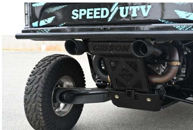
5. Lastly, install both **Tips C** to desired outlet length and tighten down. **(You may need to loosed bumper bolts and adjust bumper to get equal tip spacing.)**
