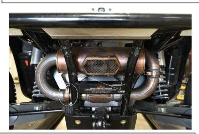
3. First, remove the factory flex pipe and the muffler by removing both V-Band clamps using a **11MM** socket and both bolts holding the muffler to the frame using a **13MM** socket.
