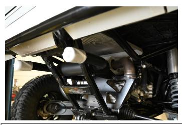
3. Then, install **Muffler Assy. A** into vehicle. Be careful as it's an extremely tight fit. Once muffler is bolted to the frame you may re-install the factory flex pipe and tighten down both V-Band Clamps. Re-use all factory hardware.
