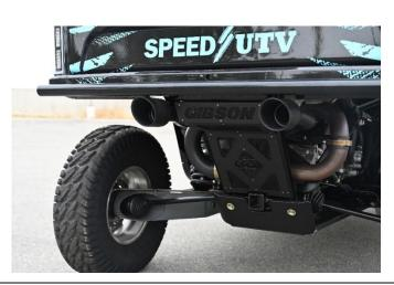
5. Lastly, install both Tips C to desired outlet length and tighten down. (You may need to loosed bumper bolts and adjust bumper to get equal tip spacing.)
