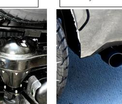
5. Install your over axle pipe and insert the hanger in to grommet and remove muffler support. Do not tighten
