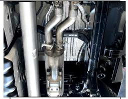
4. Using a jack or something to support the muffler install the muffler onto the head pipe. The muffler was designed to have all slip joints instated at 1.5". This can vary on each install but is a good starting point.
