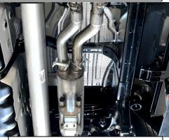
4. Using a jack or something to support the muffler install the muffler onto the head pipe. The muffler was designed to have all slip joints instated at 1.5". This can vary on each install but is a good starting point.
