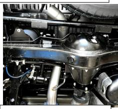
5. Install your over axle pipe and insert the hanger in to grommet and remove muffler support. Do not tighten
