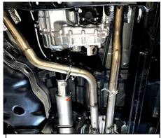
3. Install Passenger and driver Mid-pipe. Insert the hangers into the rubber grommets. Loosely tighten down because you will need to make final adjustments to find the right fit for your vehicle with the right clearance.
