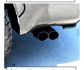
6.Install your exit pipe and exhaust tips. Now go back and adjust the kit so you have proper clearance and the muffler sits level with the frame rail, the tips were designed to have the tips 1" below the ¼ panel. Begin to tighten from the front to the back. Check clearance as parts will move.
