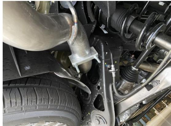
2. Lay out the exhaust on the floor so it looks like the drawing and compare parts with manual. To remove the stock exhaust, you'll need to cut it where indicated in the photo above. **(Factory rubber hanger grommet will be re-used, use wd-40 to aid in removal.)**
