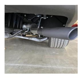
4.) Install the tip to your desired location then tighten the clamp.
