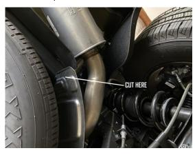
2. Lay out the exhaust on the floor so it looks like the drawing and compare parts with manual. To remove the stock exhaust, you'll need to cut it where indicated in the photo above. (Factory rubber hanger grommet will be re-used, use wd-40 to aid in removal.)
