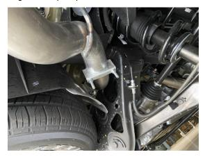
3. Install exit pipe #a onto stock pipe. Use clamp #b, do not tighten.
