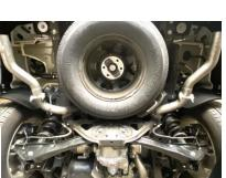
Install the Over Axle (B) **#D** onto the PS output of the First Over Axle Pipe then install Over Axle (C). Use clamps **#G** to secure pipe. Do not tighten. Next, Install the Exit Pipes **#E** with the tips pre-installed to set height, then tighten using clamps
