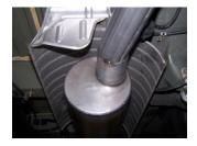
**4.** Install muffler #B onto headpipe 1½"-2" with the louvers facing towards the converter. Use a jack stand to support the muffler. Use clamp #E to secure the muffler to the headpipe. Do not tighten. Muffler inlet is looking into the louvers. Outlet of muffler will be at approximately 2 o'clock.
