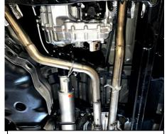
3. Install Passenger and driver Mid-pipe. Insert the hangers into the rubber grommets. Loosely tighten down because you will need to make final adjustments to find the right fit for your vehicle with the right clearance.
