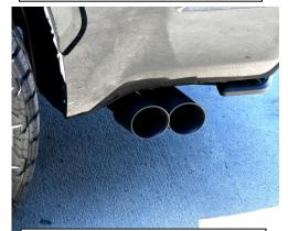
6.Install your exit pipe and exhaust tips. Now go back and adjust the kit so you have proper clearance and the muffler sits level with the frame rail, the tips were designed to have the tips 1" below the ½ panel. Begin to tighten from the front to the back. Check clearance as parts will move.
