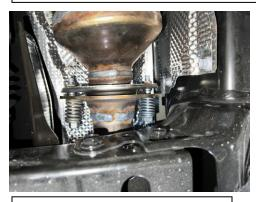
2. Install Driver side and Passenger side Head pipe onto the factory flanges. loosely tighten down the flange with the factory springs on the rear side of the Gibson Flange.
