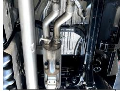
4. Using a jack or something to support the muffler install the muffler onto the head pipe. The muffler was designed to have all slip joints instated at 1.5". This can vary on each install but is a good starting point.
