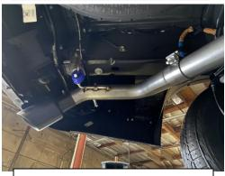
5. Install the exit pipe onto the over axle pipe and insert into rubber hangers. With exhaust loose make adjustments to find the proper tip position and clearance from all vehicle's components.
