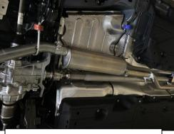
4. Install the over axle pipe into the muffler. Loosely tighten down.
