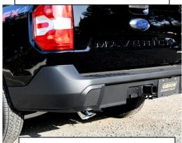
7. Be sure to check all clearance after each section has been tightened to be sure there is proper clearance. It may take 4-500 miles for your vehicle to fully adjust to the changes in exhaust flow.
