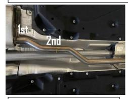
2. Please note the cut will be in the  $2^{nd}$  straight section in front of the factory muffler and is 13" from the front of the factory muffler forward.
