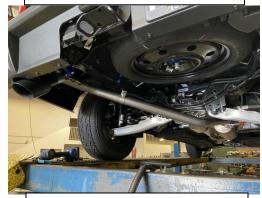
6. With proper clearance from spare tire, install the exhaust tip onto the tailpipe. The system was designed to have the tip 1" below the bumper panel of the vehicle. With the tip in your desired position begin to tighten down all clamp connections from the front head pipe back.
