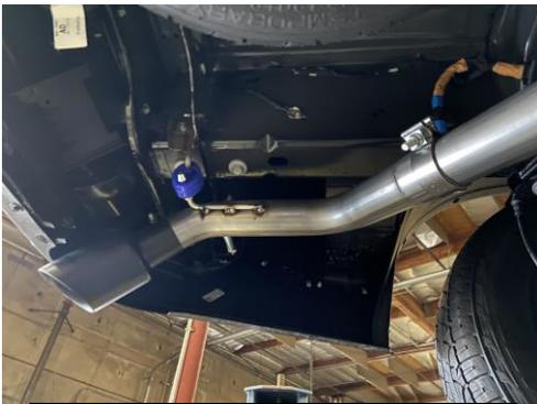
5. Install the exit pipe onto the over axle pipe and insert into rubber hangers. With exhaust loose make adjustments to find the proper tip position and clearance from all vehicle's components.
