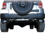
4. Install tips. Clamp down. When you have everything in place, firmly tighten all bolts and clamps down securely. Inspect all fasteners after 25-50 miles of operation and retighten as necessary.
