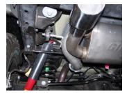
3. Install muffler assembly #A onto stock pipe. Insert welded hangers into rubber grommets. Use clamp #B to secure.
