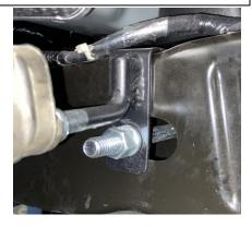
2. Install Headpipe Item # A onto the factory flange using factory bolts. Install muffler with louvers opening towards the rear of the vehicle. Facing them forward will reduce sound levels and quality of sound.
