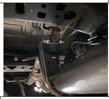
7 After your vehicle has gone through a few heat cycles re torque all your clamps and double check fitment. Use soap and water to clean your black ceramic coated stainless steel tips.
