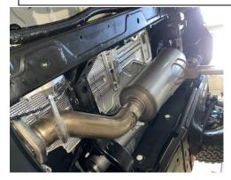
2. Install Headpipe Item # A onto the factory flange using factory bolts. Install muffler with louvers opening towards the rear of the vehicle. Facing them forward will reduce sound levels and quality of sound.
