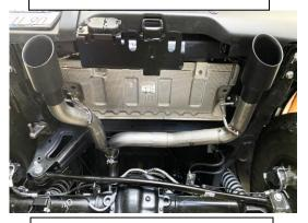
6. Install the tips. They were designed to have a .75" of an inch clearance from the bumper. Adjust pipes and all connections to find that perfect fit. Begin to tighten all connections from the front to the back. Double check you tip exit locations after each connection is tight.
