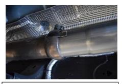
2. Remove clamp from factory head pipe using a small flathead screwdriver to bend up the retaining clip and then install onto new head pipe (Item A). Next, install head pipe and tighten with allowance for adjustment.
