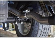
6. Install supplied 2-1/2" band clamp(Item I) onto the inlet side of both the Driver and Passenger side exit pipes(Item F) and install them onto the outlets of each over-axle pipe. Tighten both clamps with allowance for adjustment.
