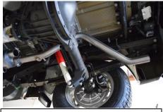
4. Before install of (Item C) install supplied rubber hanger onto factory hanger mount (see picture). Install supplied 2-1/2" band clamp (Item I) onto inlet side of passenger side over-axle pipe (Item C) and install onto outlet of muffler. Install hanger into factory rubber grommet hanger. Tighten with allowance for adjustment
