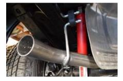
5. Before install of item E. install Driver side hanger bracket(Item G) as shown in picture. Install supplied 2-1/2" band clamp(Item I) onto the inlet side of the driver side over-axle pipe A(Item D) and install onto outlet of muffler. Install hanger into factory rubber grommet hanger. Next install another 2-1/2" band clamp(Item I) onto the inlet side of driver side overaxle pipe B(Item E) and install onto outlet of Item D. Tighten both clamps with allowance for adjustment
