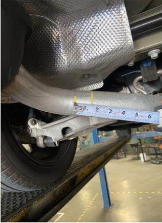
1. First you'll need to cut both tailpipes 1.5" from the beginning of each straight closest to the muffler, the cuts are marked in this photo. **(BE SURE YOU CUT CORRECTLY).**
