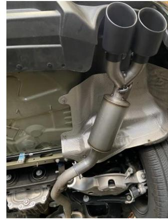
3. Now begin installing the passenger side muffler assy. #B using another clamp #C. Once finished you may install all tips #D onto the exits and tighten the exhaust.
