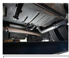
5 With everything in place and sitting with proper clearance begin to tighten the clamps from the front to the back. Tighten each side evenly. We recommend using an impact wrench.
