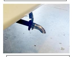
6. To Install the Generator turn down tip. Simply hold the tip up to your factory exhaust and mark the end of the tip. Add 1.5" to the mark towards the end of the exhaust and cut. Be sure the tip still extends past your body panel 1.5".
