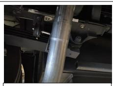
3. Install the overaxle pipe into the muffler outlet no less then 1.5". Please note when using the clamp it needs to be place to the furthest point of the muffler outlet to grab both pipes.
