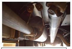
2. Install the muffler onto the factory head pipe and slide into the factory rubber grommets. Do not tighten.
