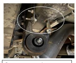
5. You may need to use the provided drop hanger to find the right height. If so, you will un bolt the factory hanger and use the kit to drop it down with the provided hardware.
