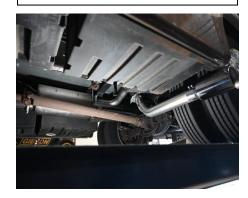
6 With everything in place and sitting with proper clearance begin to tighten the clamps from the front to the back. Tighten each side evenly. We recommend using an impact wrench.
