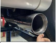
4. Slide the tip onto the Gibson exit pipe. Then install it onto the overaxle pipe, You will do this to help determine the correct height. The tip should be no closer than 1.5" to your RV body panel and stick out no less 1.5" Do not tighten
