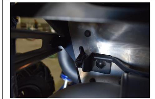
**2.** Remove the factory exhaust by un-bolting the factory rear shield that covers the muffler. You will re-use the hardware for the Gibson install. Disconnect the 2 factory springs and unbolt the factory exhaust. **Do not damage the factory exhaust gasket.** You will re-use this gasket. Remove both lower aluminum brackets that hold the factory exhaust shield. They will not be used with this kit.
