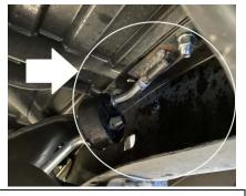
5. Install your tailpipe hanger in to the existing frame holes shown in the photo. Use the provided bolt kit and do not tighten.
