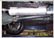
3. Install the muffler onto your head pipe. Be sure all slip joints are in a minimum of 1.5". The muffler inlet will have the louvers facing forward. Do not tighten.
