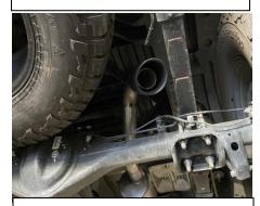
6. With proper clearance from spare tire, install the exhaust tip onto the tailpipe. With the tip in your desired position begin to tighten down all clamp connections from the front head pipe back.
