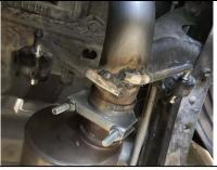
4. Install the over axle pipe into the muffler outlet a minimum of 1.5" and insert the hangers into the rubber grommets. The muffler outlet will be positioned closely to 2:00 o clock. Do not tighten down.
