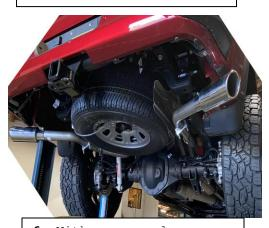
6. With proper clearance from spare tire, install the exhaust tip onto the tailpipe. The system was designed to have the tip 1" below the quarter panel of the vehicle. Note you can adjust the tip position inward or outward with rotation of the exit pipes.
