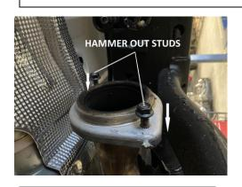
2 First you'll need to unbolt the factory flange and remove the exhaust. Next, hammer out the studs protruding from the factory flange, then install head pipe #A and tighten with allowance for adjustment using Bolt Kit #M.
