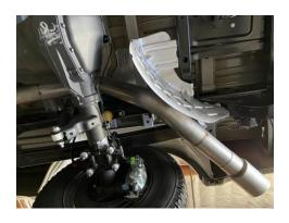
**5.** Finally, over axle pipe #C can be installed using the Band Clamp #E. Once the over axle pipe is in you may install the Tip to your desired wants. (Tighten all clamps working from front to back.)
