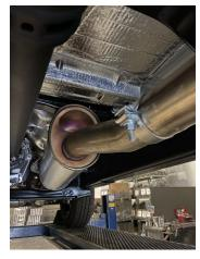
2. TO REMOVE YOUR STOCK EXHAUST, REMOVE IT FROM THE CLAMP LOCATED JUST IN FRONT OF THE RESONATOR. REMOVE HANGERS FROM RUBBER GROMMETS, USE WD-40 TO AID IN REMOVAL, LEAVE GROMMETS IN PLACE.
