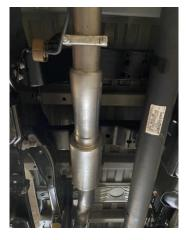
4. INSTALL MUFFLER #B ONTO HEADPIPE, USE CLAMP #D TO SECURE MUFFLER TO HEADPIPE. DO NOT TIGHTEN. USE A JACK STAND TO HOLD UP THE MUFFLER. OUTLETS SHOULD BE LEVEL.
