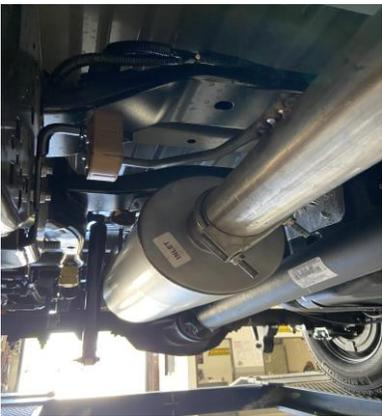
INSTALL MUFFLER # H ONTO HEADPIPE, USE CLAMP #D TO SECURE MUFFLER TO HEADPIPE. DO NOT TIGHTEN. USE A JACK STAND TO HOLD UP THE MUFFLER. OUTLETS SHOULD BE LEVEL.
