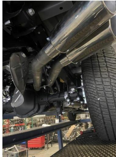
INSTALL DRIVERS SIDE TAILPIPE #C INTO THE MUFFLER, INSERT HANGERS INTO RUBBER GROMMETS, USE CLAMP #E TO SECURE PIPE TO MUFFLER. DO NOT TIGHTEN. THE TAB ON THIS PIPE SHOULD GO ON BOTTOM OF PASSENGER SIDE PIPE USE BOLT KIT #G TO SECURE TOGETHER.
