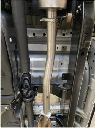
INSTALL HEADPIPE #A ONTO STOCK PIPE BEHIND RESONATOR. INSERT WELDED HANGER INTO RUBBER GROMMET. USE CLAMP #D PROVIDED TO SECURE. DO NOT TIGHTEN.
