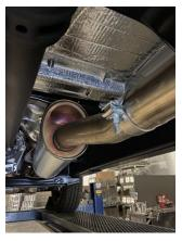
TO REMOVE YOUR STOCK EXHAUST, REMOVE IT FROM THE CLAMP LOCATED JUST IN FRONT OF THE RESONATOR. REMOVE HANGERS FROM RUBBER GROMMETS, USE WD-40 TO AID IN REMOVAL, LEAVE GROMMETS IN PLACE.
