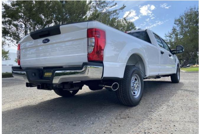
5. Now you may install the Over Axle Pipe #B into the muffler using Clamp #C. Then install the Tip onto the over axle to your desired location and tighten all clamps working front to back.
