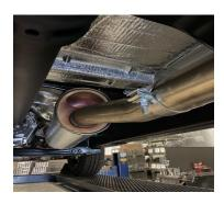
2. To remove the stock exhaust loosen the clamp from the back of the resonator. Then remove the spare tire and heat shield to aid in removal. Disengage the welded hanger using WD-40 from the OEM rubber grommets. Do not damage or remove the rubber grommets as you will reuse it to mount your new system.
