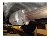
TO REMOVE YOUR STOCK EXHAUST, CUT THE SYSTEM IN HALF THEN UN-BOLT IT FROM THE FLANGE LOCATED JUST IN FRONT OF THE MUFFLER, REMOVE HANGERS FROM RUBBER GROMMETS, USE WD-40 TO AID IN REMOVAL, LEAVE GROMMETS IN PLACE. REMOVE HEAT SHEILD ABOUVE FACTORY MUFFLER AS IT WILL NOT BE NEEDED.
