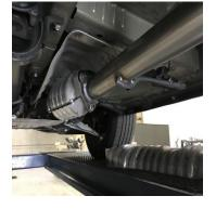
INSTALL HEADPIPE #B ONTO STOCK FLANGE. INSERT WELDED HANGERS INTO RUBBER GROMMET.
