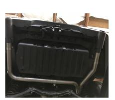
INSTALL DRIVERS SIDE EXIT PIPE # D ONTO PIPE #C 1  $\frac{1}{2}$ " TO 2"., USE CLAMP #F TO SECURE PIPE TO ASSY. DO NOT TIGHTEN FULLY. INSTALL HANGER #E IN THE SAME LOCATION AS THE OTHER SIDE, USE CLAMP #F TO HOLD PIPE IN PLACE.
