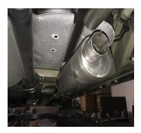
INSTALL MUFFLER # A ONTO HEADPIPE  $1\frac{1}{2}$ " TO 2". USE CLAMP # F TO SECURE MUFFLER TO HEADPIPE. DO NOT TIGHTEN. USE A JACK STAND TO HOLD UP THE MUFFLER. OUTLET SHOULD BE CLOCKED AT 9 O'CLOCK
