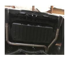
INSTALL DRIVERS SIDE EXIT PIPE # D ONTO PIPE #C 1 ½" TO 2"., USE CLAMP #F TO SECURE PIPE TO ASSY. DO NOT TIGHTEN FULLY.
