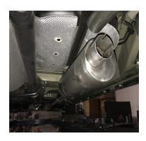
INSTALL MUFFLER # A ONTO HEADPIPE 1 ½" TO 2". USE CLAMP # F TO SECURE MUFFLER TO HEADPIPE. DO NOT TIGHTEN. USE A JACK STAND TO HOLD UP THE MUFFLER. OUTLET SHOULD BE CLOCKED AT 9 O'CLOCK
