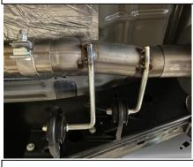
2. INSTALL HEADPIPE #A ONTO STOCK FLANGE. INSERT WELDED HANGER INTO RUBBER GROMMET. USE BOLT KIT PROVIDED TO SECURE. DO NOT TIGHTEN
