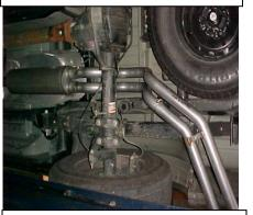
6. THE TAB ON DRIVER SIDE PIPE SHOULD GO UNDERNEATH THE PASSENGER SIDE PIPE TAB. USE BOLT KIT # H TO SECURE TOGETHER.
