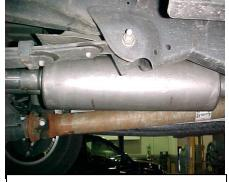
3 INSTALL MUFFLER # B ONTO HEADPIPE 1 ½″ TO 2″. USE CLAMP # F TO SECURE MUFFLER TO HEADPIPE. DO NOT TIGHTEN. USE A JACK
