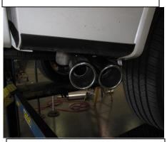
7. Be sure to check all clearance after each section has been tightened to be sure there is proper clearance. It may take 4-500 miles for your vehicle to fully adjust to the changes in exhaust flow.
