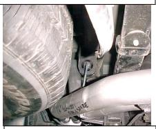
4 INSTALL PASS. SIDE TAILPIPE # C INTO MUFFLER 1 ½" TO 2". INSERT HANGER INTO RUBBER GROMMET, USE CLAMP # G TO SECURE PIPE TO MUFFLER. DO NOT TIGHTEN.
