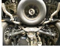
Re install spare tire and heat shield. Position all pipes and double check all connections prior to tightening clamps.
