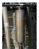
Install muffler onto head pipe **#A** 1-1/2" to 2" with the louvers facing towards the converter. Use a jack stand to support the muffler. Use clamp **#H** to the secure the muffler to the head pipe. Do not tighten
